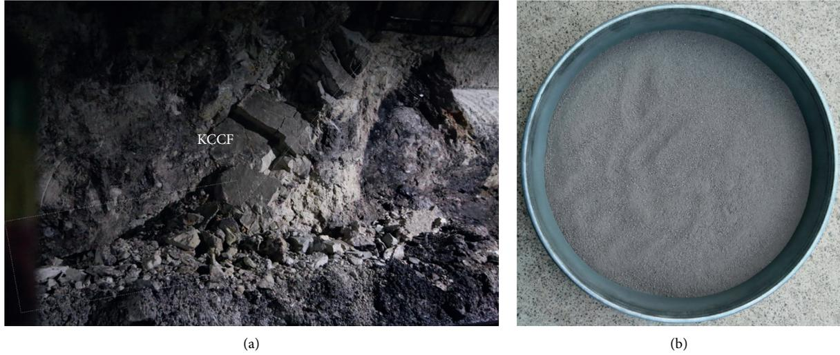
FIGURE 1: Test filling material of KCC X3. (a) KCC X3 at Sima coal mine. (b) Crushed and dried filling material particles.
