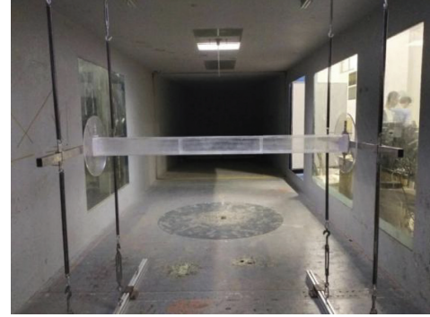
FIGURE 3: Installation of the sectional model in the wind tunnel.
