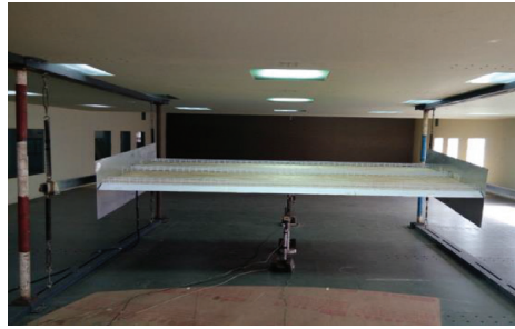
FIGURE 2: Layout of the section model wind tunnel test.
