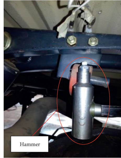
FIGURE 7: The hammer impact test of Z direction at left-front suspension.
