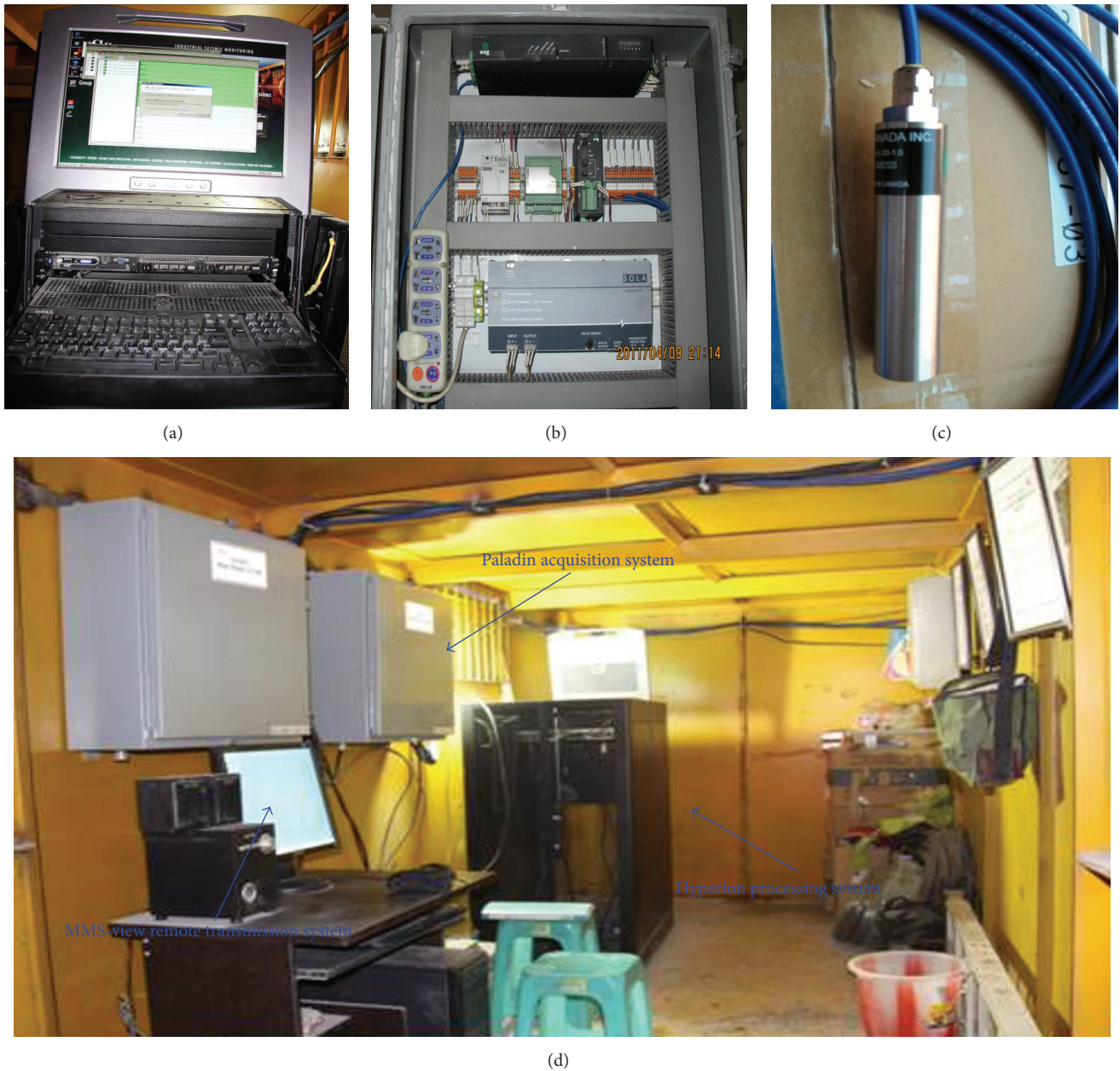
FIGURE 4: Constitution of microseismic monitoring system. (a) Hyperion digital signal processing system. (b) Paladin digital signal acquisition system. (c) Acceleration sensor. (d) Center of the site monitoring system.
