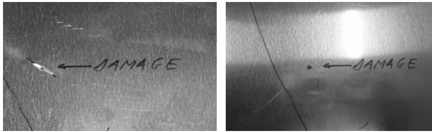
Fig. 13. Example of two types of damages created in the plate.
