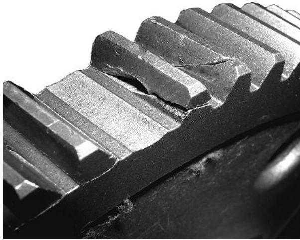
Fig. 1. Typical example of a tooth bending fatigue crack.
