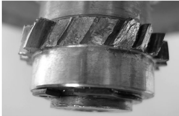
Fig. 5. Resulting fatigue damage on the test gear.
