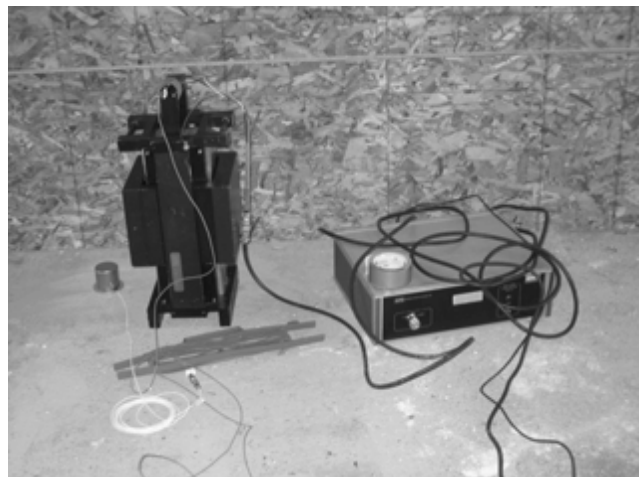
Fig. 5. Shaker, amplifier and accelerometers used for the modal testing.
