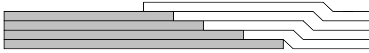
Fig. 1. Scarf joint of two composites, one in gray and the other in white.
