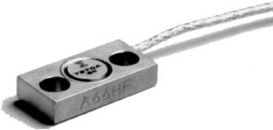
Fig. 5a. The first high-g (200,000 g) sculptured silicon accelerometer (Endevco, 1983).
