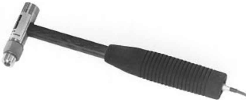
Fig. 4. The first modally tuned impulse hammer (PCB, 1972).
