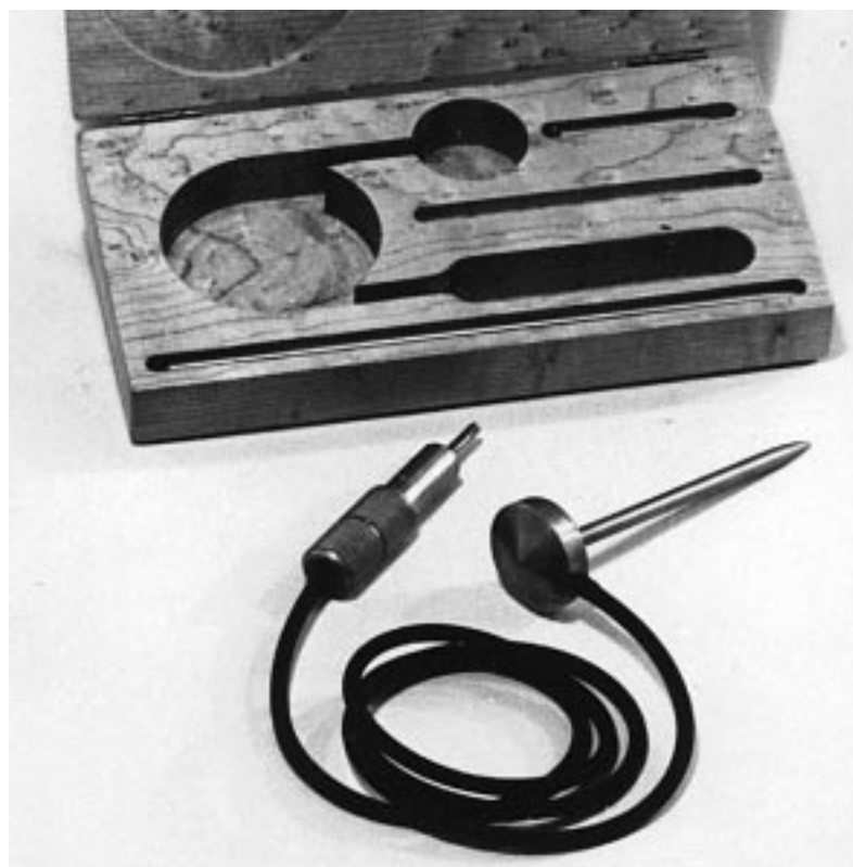
Fig. 2. The first commercial piezoelectric accelerometer (B&K, about 1943).
