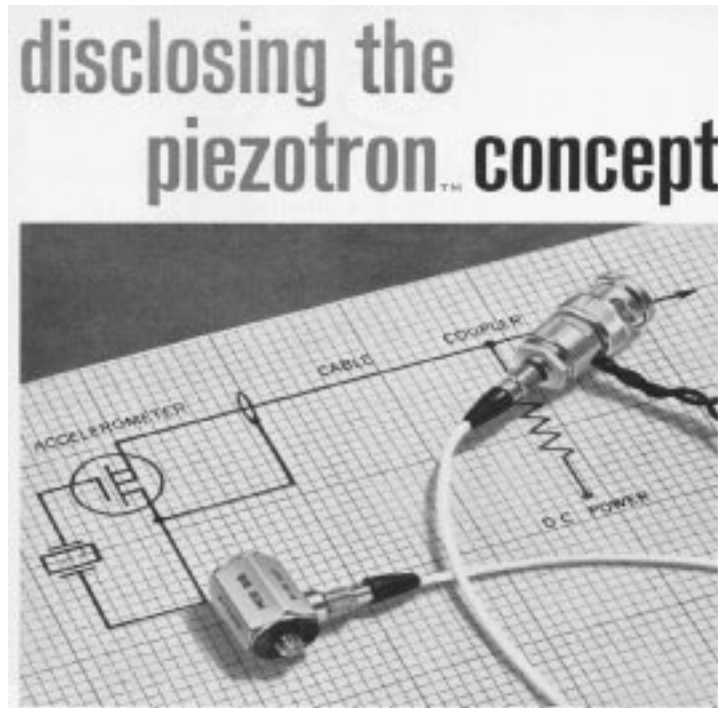
Fig. 3. The first commercial two-wire piezoelectric accelerometer with contained FET (Kistler, about 1963).
