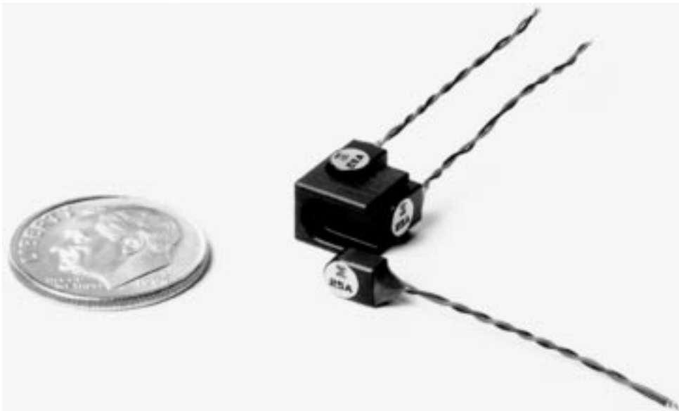
Fig. 5b. The smallest triaxial piezoelectric accelerometer with integral electronics (Endevco, about 1985).
