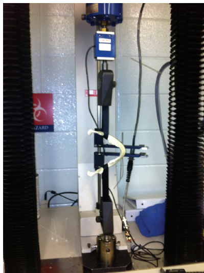
FIGURE 6: Sample positioned for mechanical testing in the Sintech 2/G servohydraulic materials testing unit.
