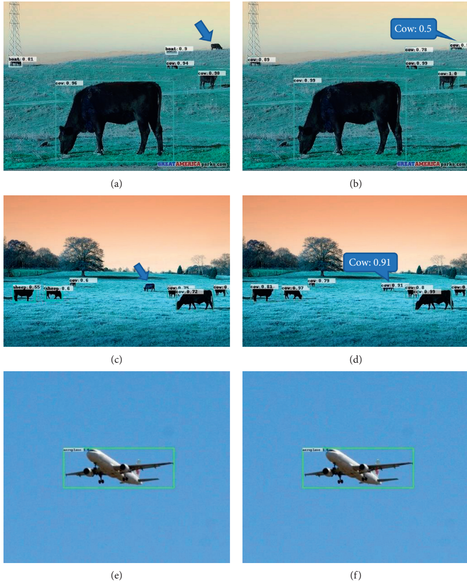
FIGURE 5: Examples of fixed weights using FPN (a) and adaptive weights using SAFPN (b). SAFPN gave large weight to high resolution feature map c_3 in (B) and (D), which helps detection of small objects. For image (F) containing a large object, SAFPN gave large weight to low resolution feature map c_5 . (a) A “cow” far in the background is not detected [w_c^2, w_c^3, w_c^4, w_c^5] = [0.5, 0.5, 0.5, 0.5] . (b) A small “cow” far in the background is detected. Smaller scales (level 2 and 3) have higher weights for this image [w_c^2, w_c^3, w_c^4, w_c^5] = [0.28, 0.34, 0.19, 0.16] . (c) Small cow near the center of image is not detected [w_c^2, w_c^3, w_c^4, w_c^5] = [0.28, 0.34, 0.19, 0.16] . (d) Small “cow” near the center of the image is detected. Smaller scales (levels 2 and 3) have higher weights for this image [w_c^2, w_c^3, w_c^4, w_c^5] = [0.31, 0.34, 0.19, 0.16] . (e) This image contains easy-to-detect large object, an airplane [w_c^2, w_c^3, w_c^4, w_c^5] = [0.5, 0.5, 0.5, 0.5] . (f) With a large object, SAFPN weighs larger scale (i.e., lowest resolution) feature map at level 5 [w_c^2, w_c^3, w_c^4, w_c^5] = [0.06, 0.08, 0.25, 0.61] .
