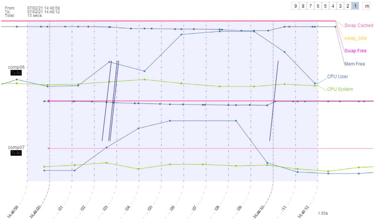
Fig. 17. The Ping Pong test magnified with "barrier" messages shown.
