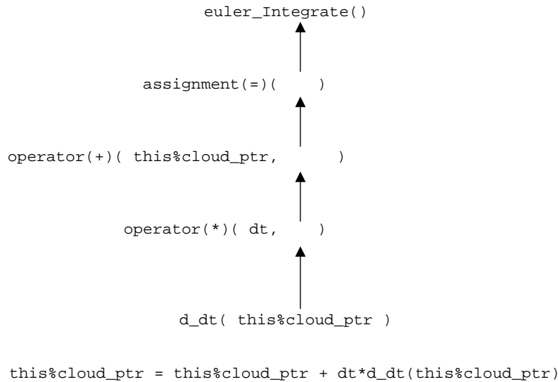
Fig. 2. Call tree for a typical euler Integrator() statement: tree (top), statement (bottom).
