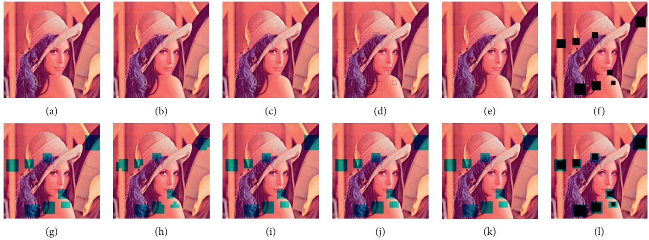
FIGURE 11: Random block attacks of the watermark Lena image: (a) blurring, (b) salt and pepper noise, (c) Gaussian noise, (d) average filter, (e) sharpening, (f) cropping, and (g–l) detection of the tampered regions of the watermarked image.
