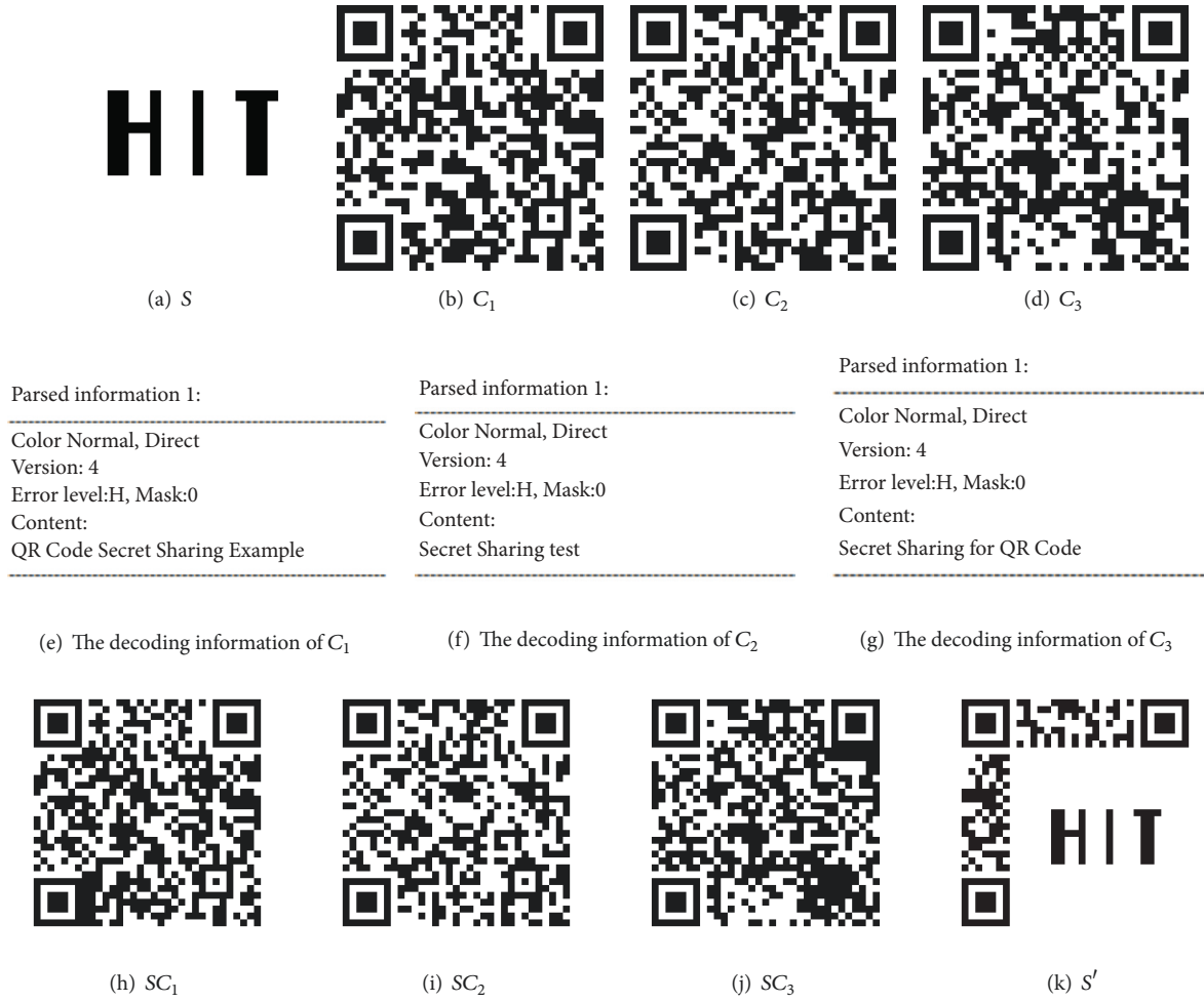
FIGURE 7: (3, 3) threshold VSS on QR code of version 4 with level of error correction H In [10].
