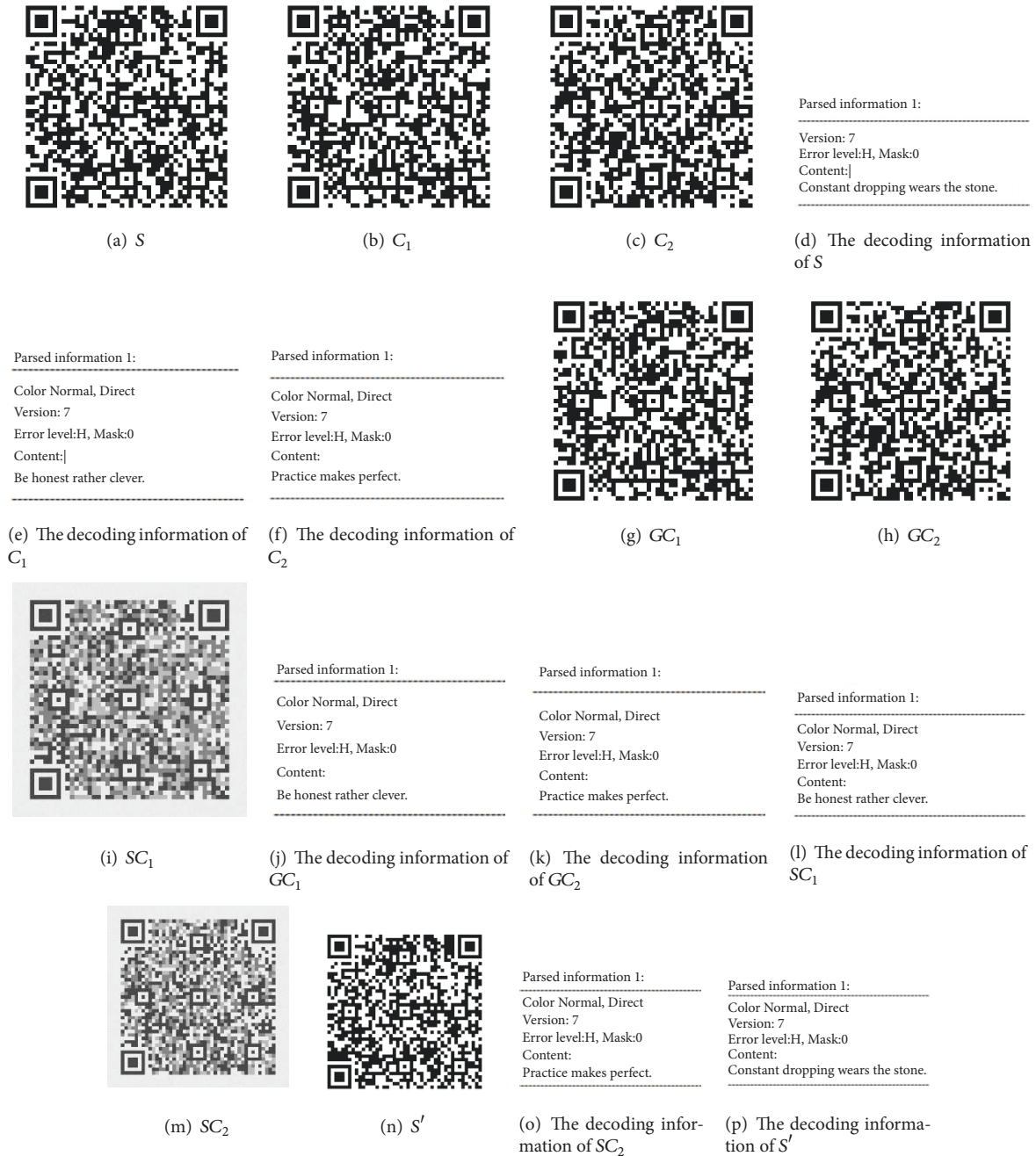
FIGURE 4: Our (2, 2) threshold XOR-based VSS on QR code of version 7 with level of error correction H.
