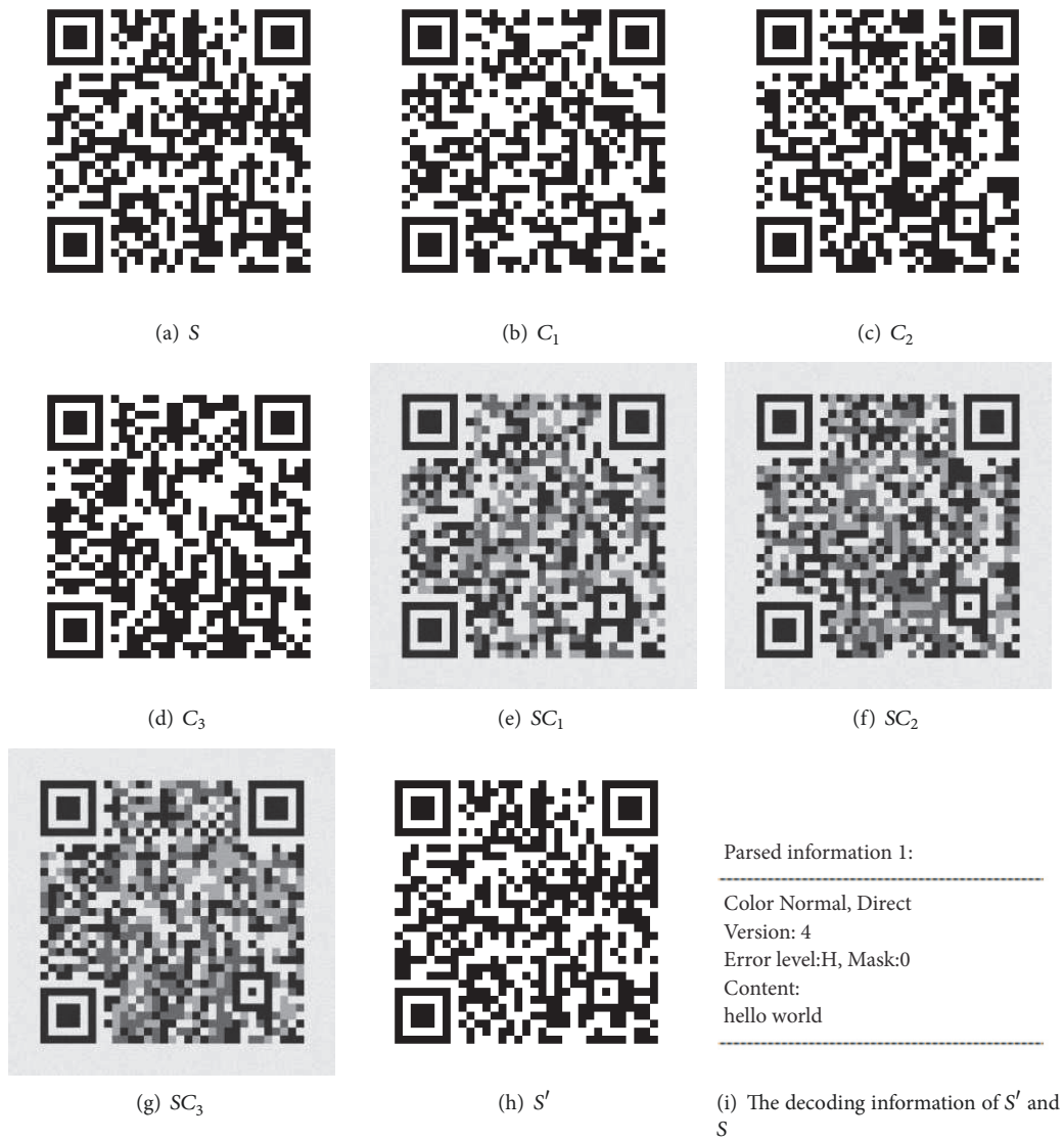
FIGURE 6: Our (3, 3) threshold XOR-based VSS on QR code of version 4 with level of error correction H.
