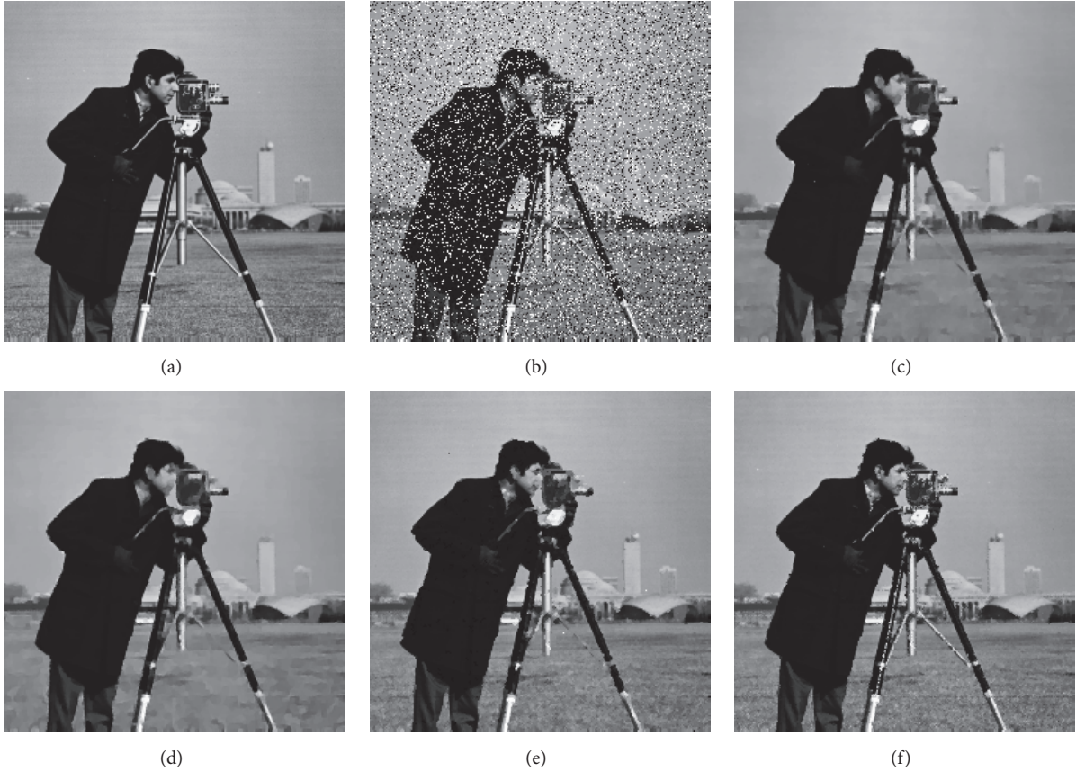
FIGURE 6: Image denoising results by different methods. (a) Original image; (b) corrupted “Cameraman” image with salt-and-pepper noise ( s = 20\% , PSNR = 12.07 dB); (c) our method ( \lambda = 1.1 , PSNR = 25.82 dB); (d) TV- L^1 ( \lambda = 1.1 , PSNR = 25.58 dB); (e) ACWMF (PSNR = 25.23 dB); (f) AMF algorithm (PSNR = 28.47 dB).
