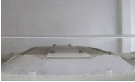
FIGURE 2: The single nozzle and the floating aluminum strip.
