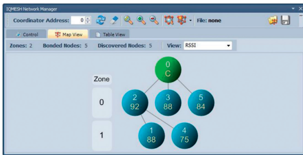
FIGURE 10: Example of network topology in IQMESH Network Manager.
