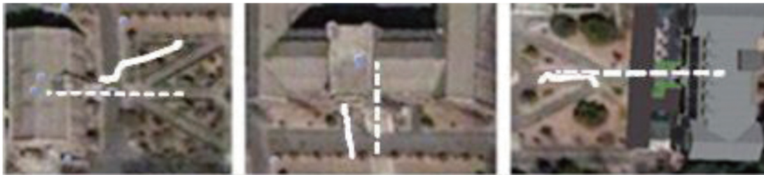
Fig. 2. GPS error near the entrance of the building. Dotted lines are real paths, and solid lines are GPS trajectories.
