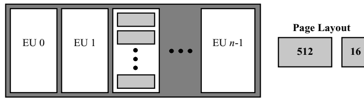
Fig. 1. The internal structure of a typical flash memory.
