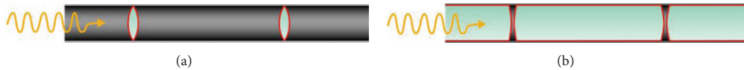
FIGURE 11: Principle of a rigid endoscope. (a) Standard rigid endoscope with high air to glass ratio. (b) Rod lens Hopkins endoscope. The reverse relation of glass to air and better coating of the lenses improves the light transmission 80-fold in comparison to the standard endoscope.
