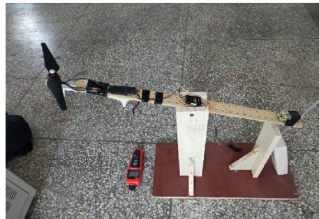
FIGURE 9: Simple lift test device.
