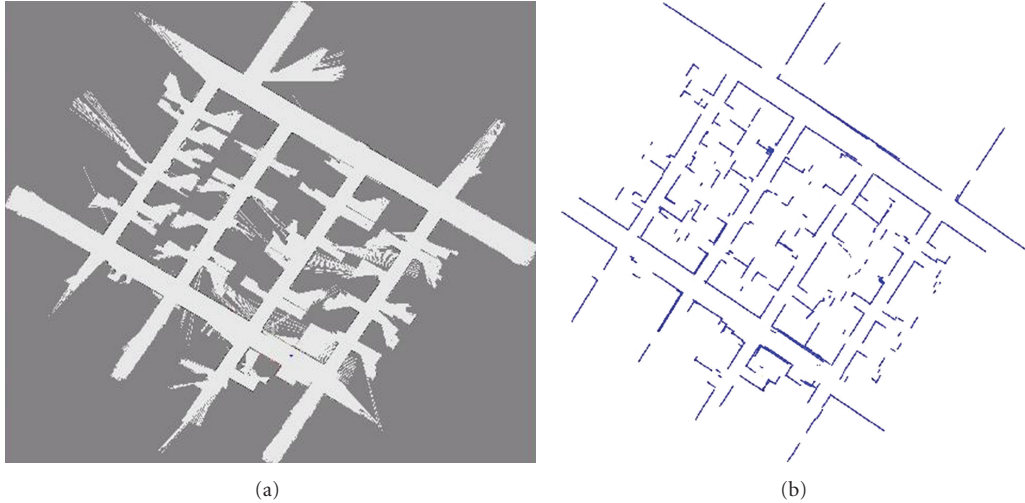
FIGURE 14: Mapping results of intel_oregon using (a) general RBPF SLAM (grid map) and (b) proposed lightweight SLAM (line segment map).
