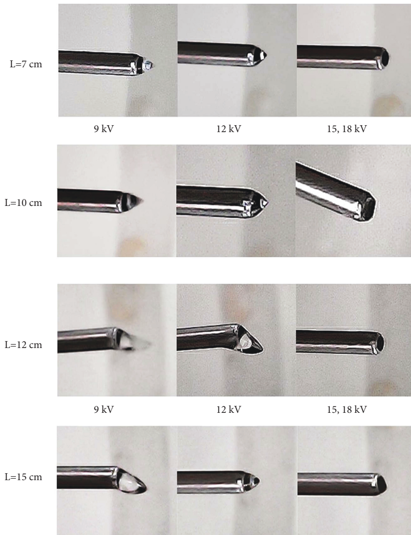
FIGURE 11: Images of the droplets of 1.5 wt.% M3 chitosan concentration in 90 wt.% acetic acid concentration changing in different voltage ( U ) and distance ( L ).
