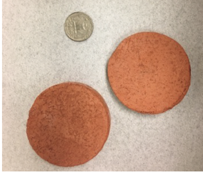
FIGURE 1: Ceramic filter disks used for laboratory testing.
