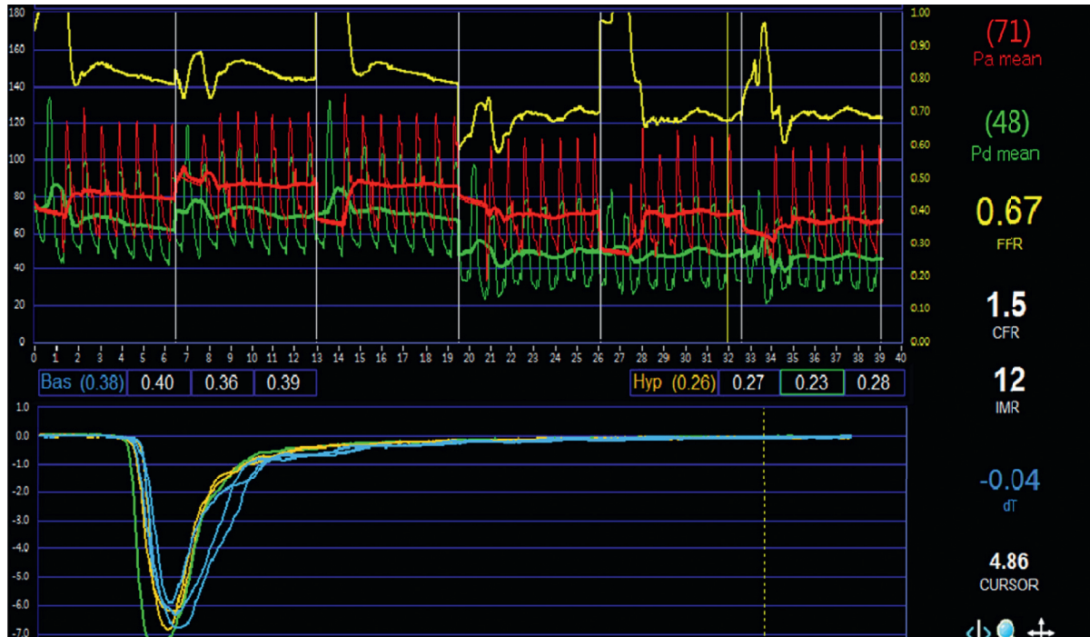
FIGURE 1: Thermodilution curves under resting conditions (yellow lines) and during hyperemia (blue lines) induced by intravenous adenosine infusion. A graphical representation of the baseline and hyperemia (seconds) thermodilution curves is seen in the catheterization lab at the time of percutaneous coronary intervention that was displayed on the RADI analyzer (Radi Medical Systems, Uppsala, Sweden).
