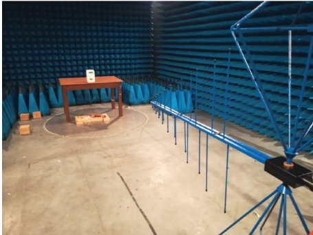
FIGURE 8: Test setup in the semianechoic room.
