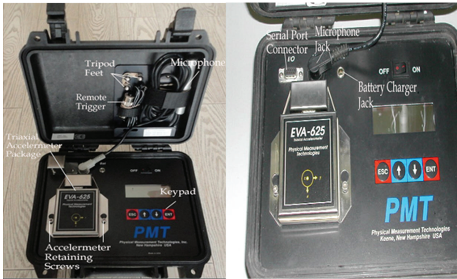
FIGURE 2: EVA-625 control and constituent parts.
