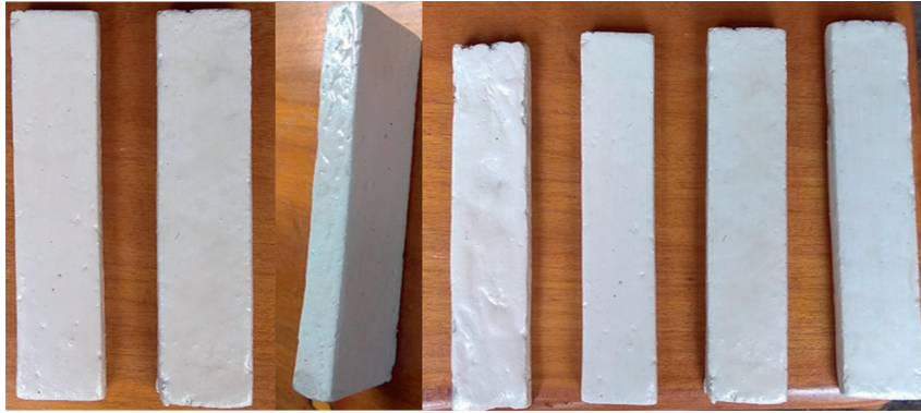
FIGURE 2: Wood sawdust-reinforced polypropylene composites.
