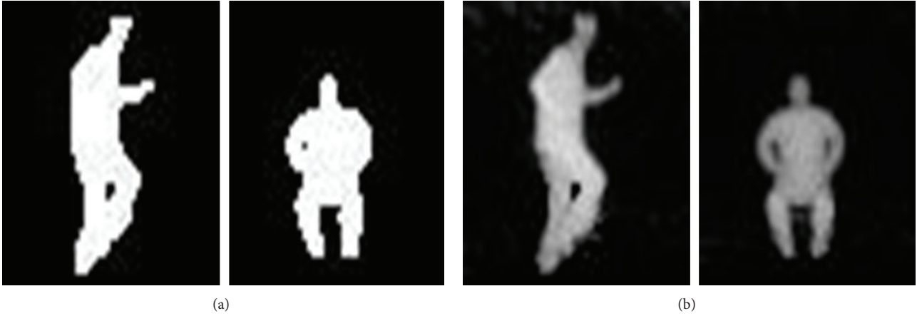
FIGURE 2: Images comparison as (a) binary silhouettes and (b) depth silhouettes of exercise and sit-down activities.
