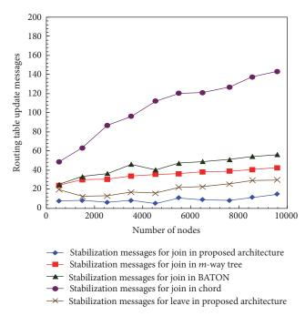
FIGURE 5: Average stabilization messages for single node join/leave.
