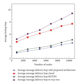
FIGURE 3: Comparison of different overlay network architectures with varying population.
