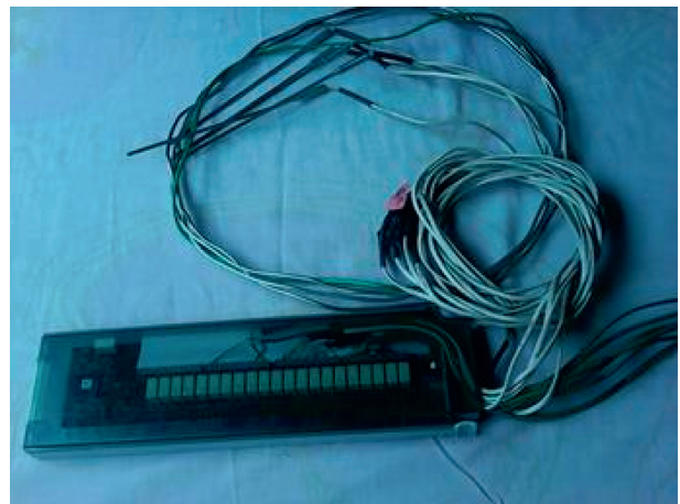
FIGURE 5: Array of 12 thermocouples connected to the 40-channel multiplexer.
