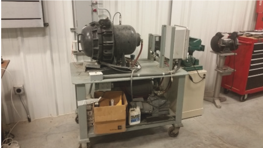
FIGURE 1: 38 L explosive chamber [9].
