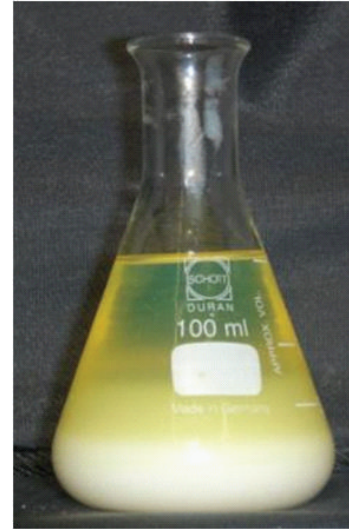
FIGURE 1: Heterogeneous mixture at room temperature, mixture of 40% fat and 60% diesel.
