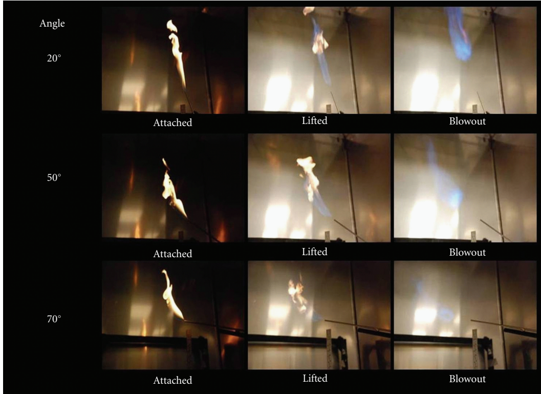
FIGURE 3: Flame states at 0.4 m/s coflow.
