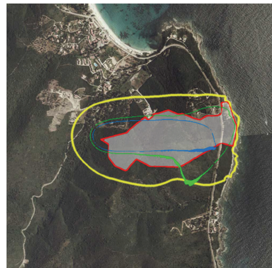
FIGURE 14: Case 2: Simulations results and observations for the Favone fire. Blue: simulated fire contour at 15:50 (after 50''), Green: simulated contour at 19:00, yellow: simulated contour at 19:00 (non coupled); Red: final observed contour of the fire.
