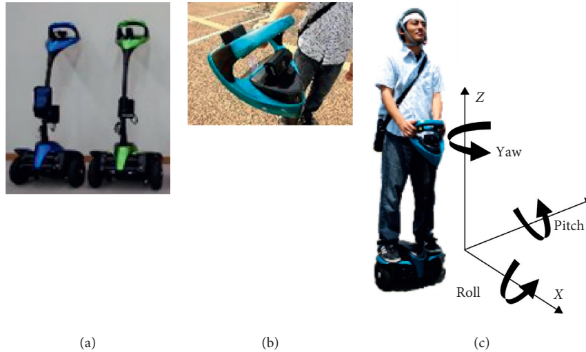
FIGURE 1: Winglet equipped with mobile sensors. The image shows the X, Y, and Z and roll, pitch, and yaw coordinate systems.
