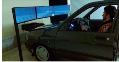
FIGURE 1: A view of the driving simulator and a driver taking the test.
