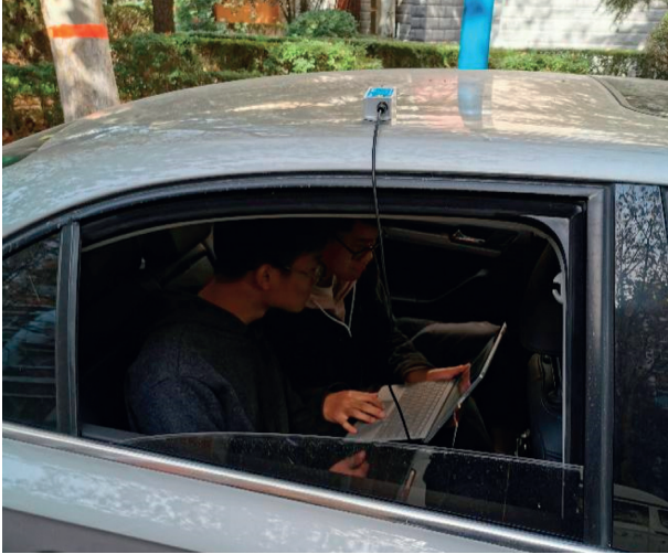
FIGURE 2: Roof-mounted acceleration sensors and data collection devices.
