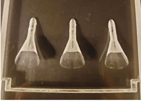
FIGURE 6: Machined test piece of \theta = 21^\circ before testing.
