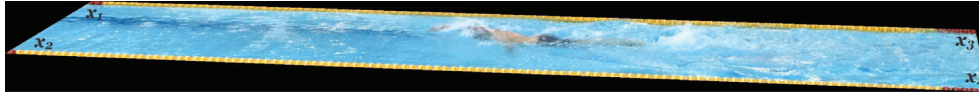
FIGURE 4: Lane extraction and mask application taking into account the four points: x_1 , x_2 , x_3 , and x_4 . The metric coordinates of these points are known and pixel coordinates are calculated using the calibration results. Swimming Championships in Limoges, France, April 2015.
