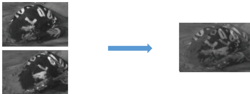
FIGURE 13: Principle of the composite filter. Left: reference images. Right: composite image which consists of a weighted summation of the two reference images.
