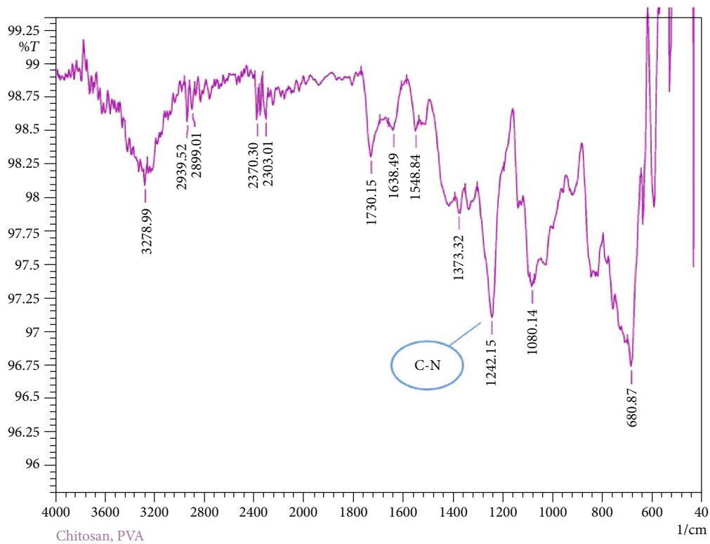
FIGURE 7: FTIR spectra of chitosan/PVA control film showing the characteristic C-N stretching peak of the chitosan polymer chain at around 1240\text{ cm}^{-1} .
