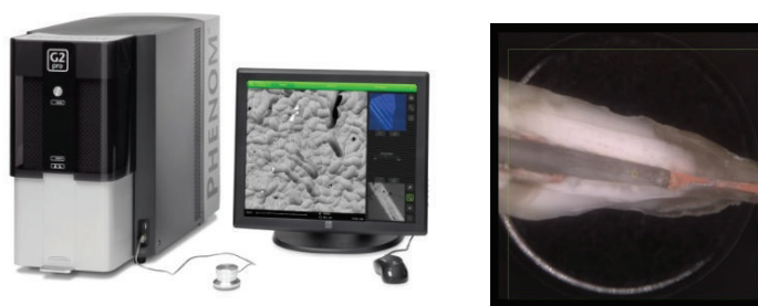
FIGURE 1: The SEM used and the low magnification image used for the observation zone determination.
