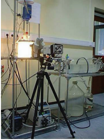
FIGURE 1: Experimental mixer-settler setup and image acquisition technique.
