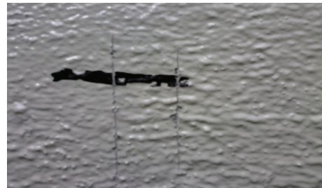
FIGURE 5: Cut test: measuring of the film thickness.
