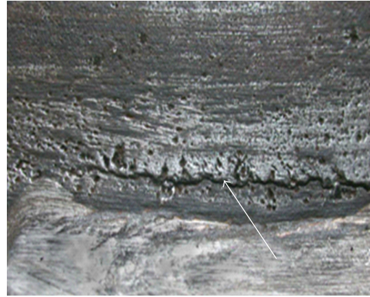
FIGURE 1: Mode 1 pitting and intergranular cracking (arrow) within the heat-affected zone of a weld deposited on incorrectly annealed base metal [13].
