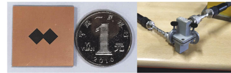
FIGURE 8: Photograph of the experimental waveguide twist and the proposed waveguide twist assigned between two mutually orthogonal waveguides.
