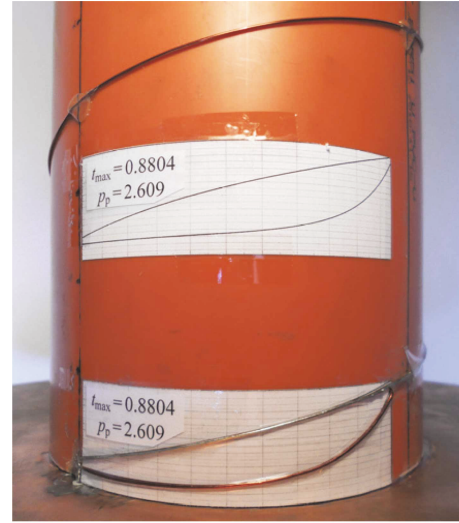
FIGURE 4: A photograph of the internally matched helix prototype. The stencil for the matching wire, preprinted on a piece of paper, is also shown.
