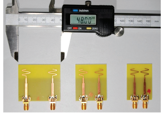
FIGURE 5: The top layer of three fabricated compact arrays. From left to right, the interelement distance is 30 mm ( 0.25\lambda ), 18 mm ( 0.15\lambda ), and 12 mm ( 0.10\lambda ) respectively.
