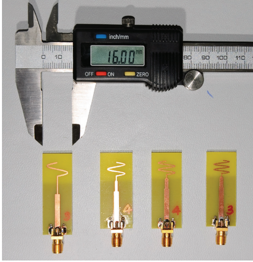
FIGURE 3: From left to right, the line-up shows iterations i = 2, 3, 4, 5 . The monopoles are mirrored against the respective optimal GNDP sizes [25–28]. The antennas were printed again on Isola IS400, so the problem with the lower permittivity persists: these monopoles were also inductive and slightly electrically larger.
